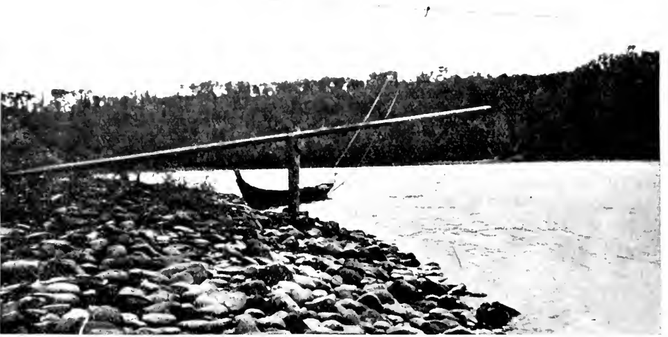
Chain gauge and measuring section, on Skeena, at Hazeiton. Measurements are made from the Indian dugout canoe shown in the foreground, points of observation being marked by a tag line.
