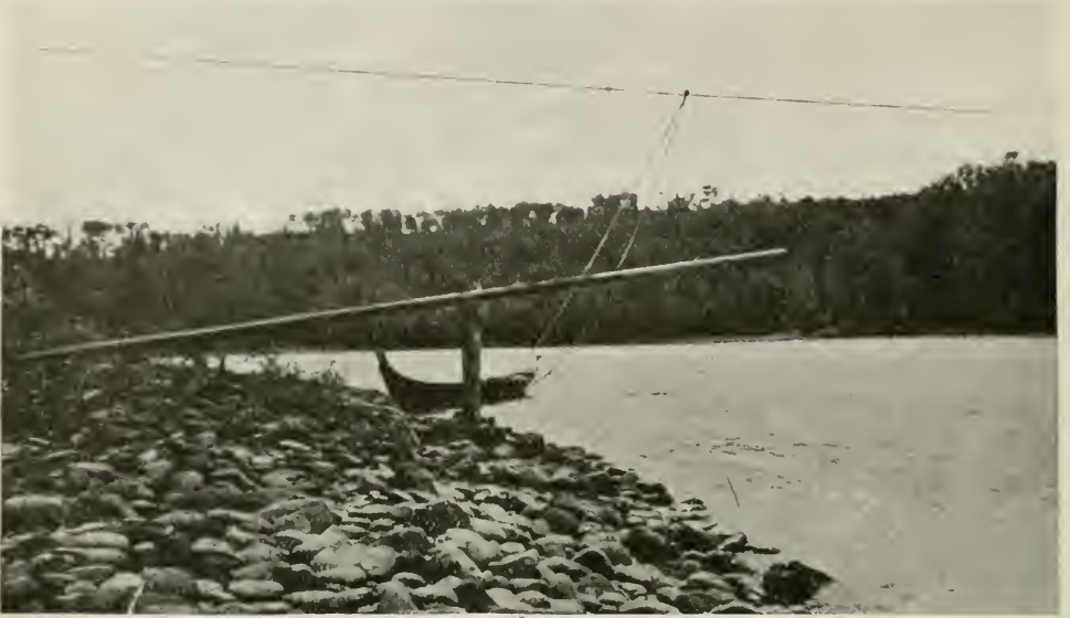
Chain gauge and measuring section, on Skeena, at Hazeiton. Measurements are made from the Indian dugout canoe shown in the foreground, points of observation being marked by a tag line.
