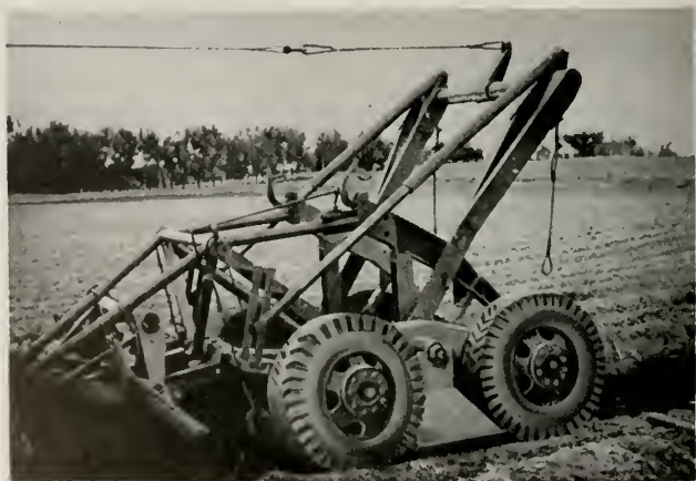
Large pneumatic tires fore and aft replace the usual caterpillar tracks on this winch-loading cable-reel trailer
