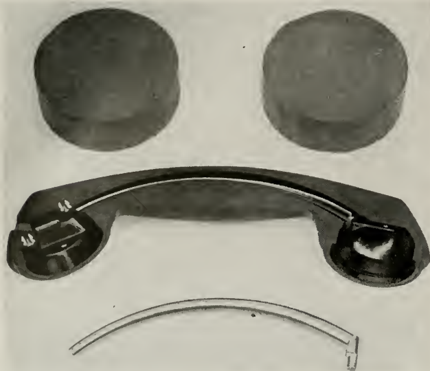
Out of these components will come a hand telephone. Top to bottom: plastic pre-forms, half section of molded handle, and core
