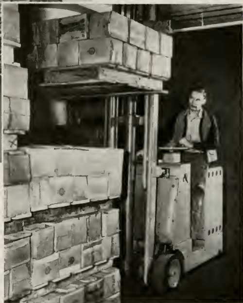
Above: "Palletization"—the use of wooden pallets and fork trucks—makes it feasible to use vertical space for storage. Right: A fork truck lifts a pallet of material for stacking. Long metal arms attached to the front of the lift truck fit inside the wooden pallet, so that pallet and load can be moved about or can be raised to as much as 14 feet above the floor
