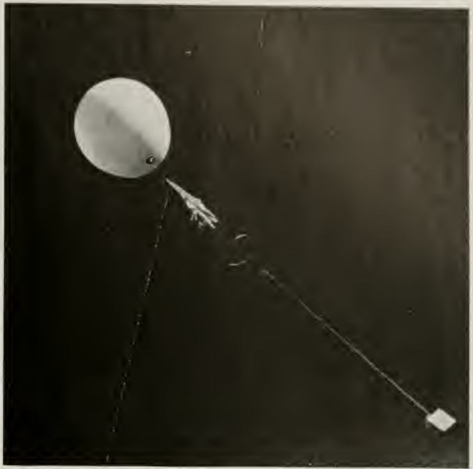
This balloon is carrying instruments aloft which will radio their records of upper air conditions to observers on the ground
