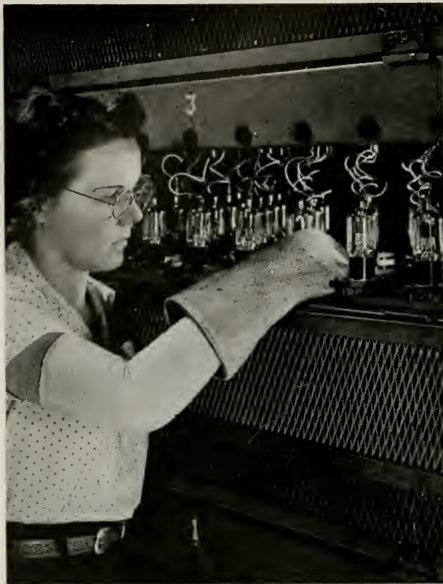
Vacuum tubes with plastic bases are placed in aging racks, where they are stabilized and tested
