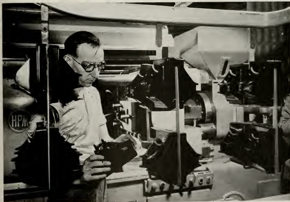
Combined-set bases travel by conveyor to the next process after being removed from the injection molding machine
