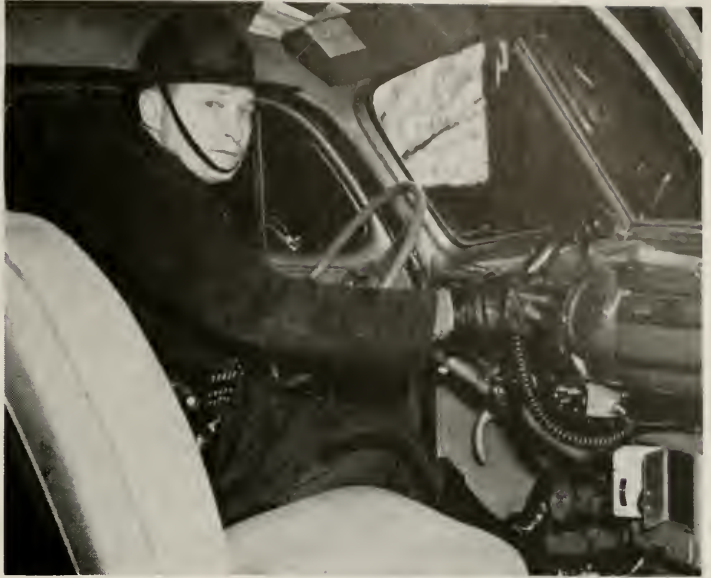
A Pennsylvania State Police patrolman reaches for the radio-telephone with which his patrol car is equipped
