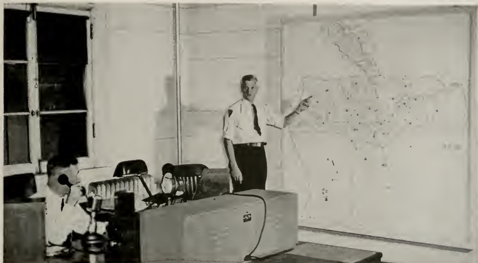
The radiotelephone dispatching layout of the Newark, N. J., municipal police. The officer at the right is pointing to the lamps on the wall map, each of which represents a radio-equipped patrol car and indicates its status
