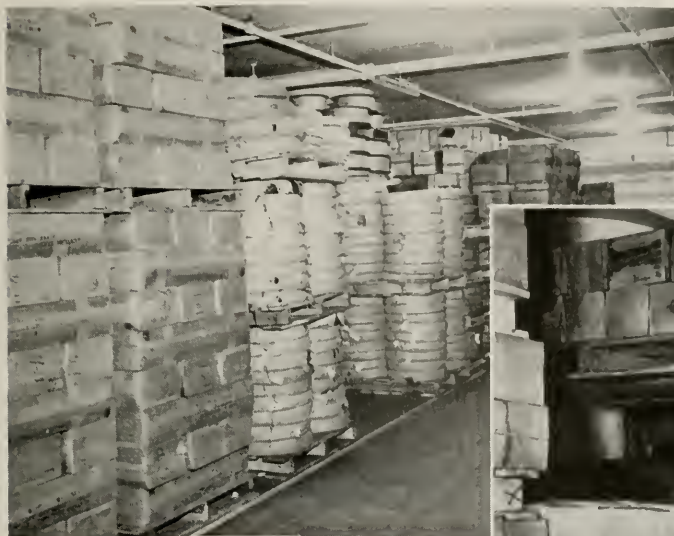
Above: "Palletization"—the use of wooden pallets and fork trucks—makes it feasible to use vertical space for storage. Right: A fork truck lifts a pallet of material for stacking. Long metal arms attached to the front of the lift truck fit inside the wooden pallet, so that pallet and load can be moved about or can be raised to as much as 14 feet above the floor
