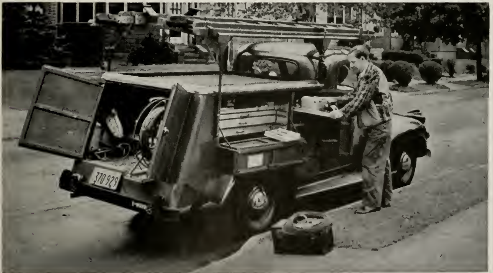
Interior arrangements in the recently developed installation truck body. With certain modification, this same body is used for a repeater-station service truck
