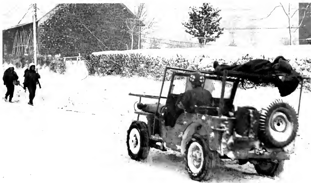
WORKHORSES OF BATTLEFIELD EVACUATION. Much of the work for transporting casualties fell to the jeep, fitted with brackets for carrying litters. When these sturdy vehicles bogged down in mud and heavy snow, medics switched to the tracked M-29 Weasel.
