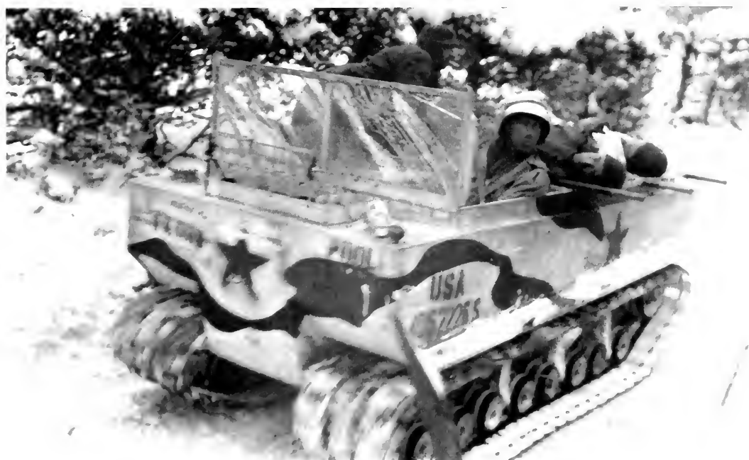
WORKHORSES OF BATTLEFIELD EVACUATION. Much of the work for transporting casualties fell to the jeep, fitted with brackets for carrying litters. When these sturdy vehicles bogged down in mud and heavy snow, medics switched to the tracked M-29 Weasel.
